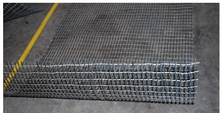
The project's FRCM system used a unidirectional carbon fiber grid (shown) along with a bidirectional grid, embedded in a portland cement-based mortar.
